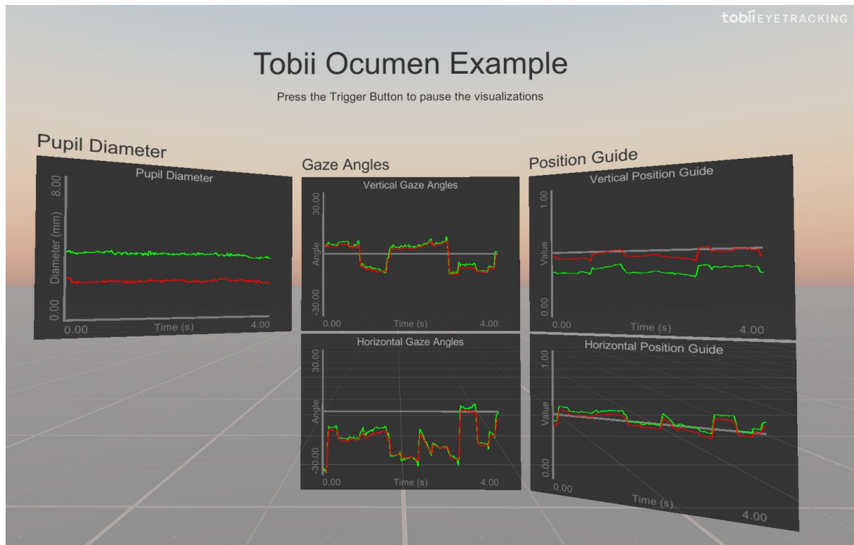
Figure 30: Example of eye-tracking indicators (pupil diameter, gaze angles, position guide), left eye is red, right eye in green © Tobii
